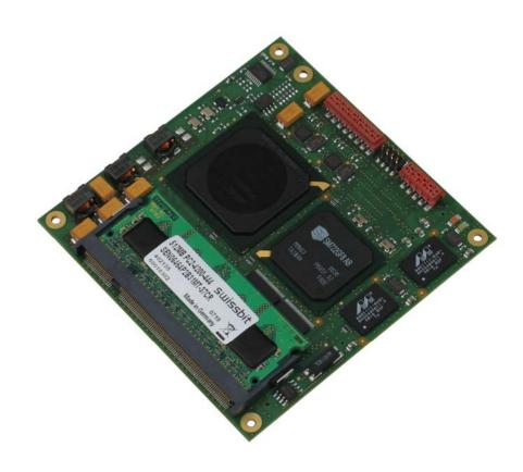
**XCOM-9460** is a highly integrated solution specially designed to meet PICMG COM.0 standard requirements. It features a low-power high-performance PowerPC processor in COM Express Compact form factor, only 95x95 mm
